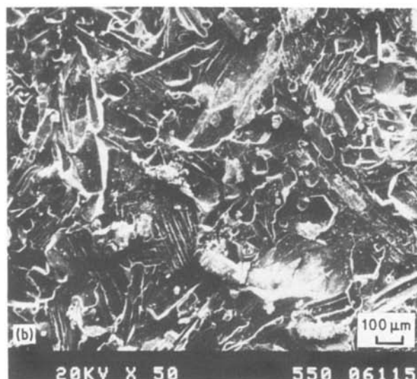
Figure 15 (a) Edge and (b) centre portions of PU films sites removed from zinc phosphate precoat surfaces after exposure for 30 days in acidic solution at 80° C. Intensity counts per 50 sec: (a) phosphorus, 549; zinc, 263; (b) phosphorus, 394; zinc, 230. Intensity ratio phosphorus: zinc, (a) 2.09; (b) 1.71.
